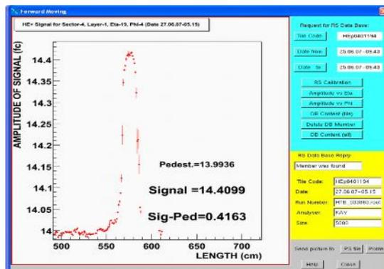
Scintillator brightening in magnetic field
