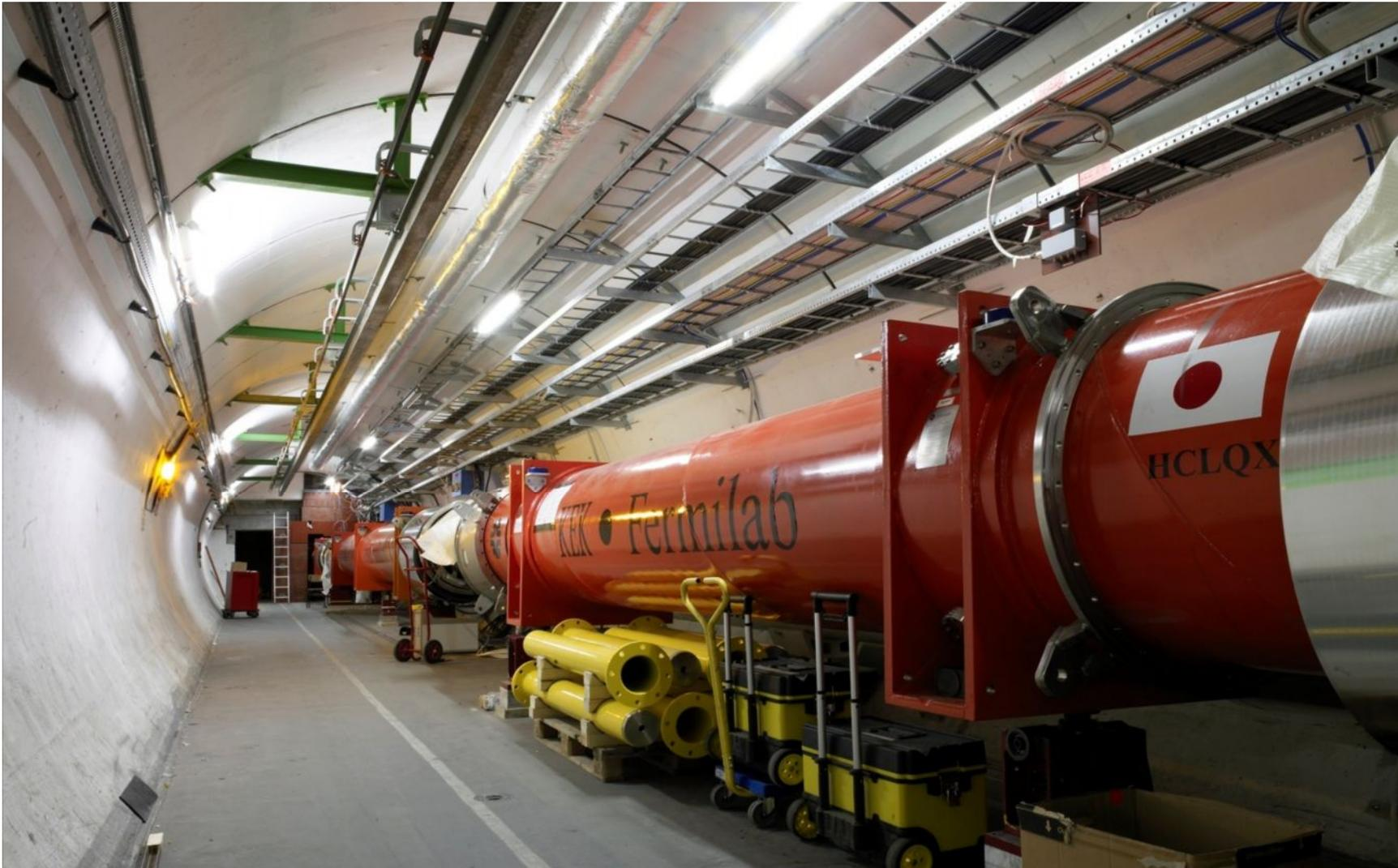
Special quadrupole magnets ('Inner Triplets') are focusing the particle beams to reach highest densities ('luminosity') at their interaction point in the centre of the experiments
