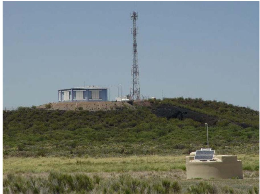
Figure 2: The Pierre Auger Observatory is a hybrid detector. On the hill is one of the 4 Fluorescence Detector buildings and communications tower. In the bottom foreground is one of the 1,600 Surface Detectors – water tanks (12,000 liter), each tank is separated from each of its neighbors by 1.5 kilometers.
