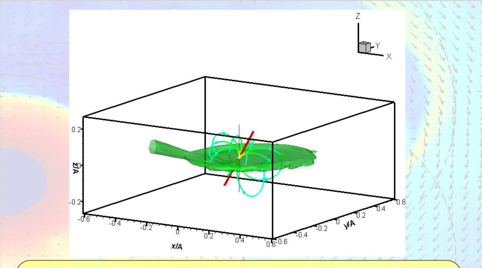
The moderate magnetic field of the accretor does not destroy the flow structure, while basic characteristics of the accretion disc change. For example, the accretion rate approximately doubles, the characteristic density decreases by roughly an order of magnitude, and thickness of the disc increases by factor of 2.
