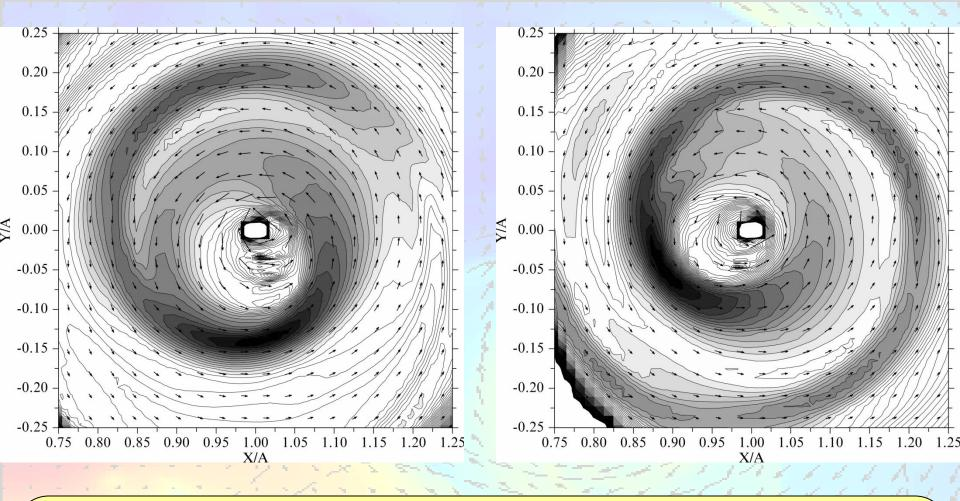
This figure shows a zoom of the density distribution and velocity vectors in the inner part of the disc for two moments of time. It is seen that the inner spiral wave rotates in the retrograde direction. Analysis of computational results shows that the wave moves in a rigid body mode with the period that is dozens times longer than the orbital one.
